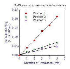
Image 1. RadChemDosi™ is an effective way to measure dose rate for ionizing radiation. In addition to calibrating the dose rate at each position in a radiation chamber periodically, it can also be used to measure the dose rate in each well of a 6 and 24 wells plate. Measurment of gamma dose rate with in 6 well plates. Dose Rate with the turntable on: Position 2- 360.28rads/min or 3.60Gy/min for each well. y=0.013x+0.000 r2=1.000 (each).
